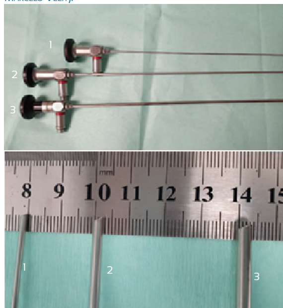
FIGURE 2. (A) OVERVIEW OF (1) 2 MM, (2) 2,9 MM AND (3) Y 4 MM OPTICS. (B) CLOSE-UP OF OPTICS IN FIGURE A. (IMAGE COURTESY DR. MARCELO VELIT).
